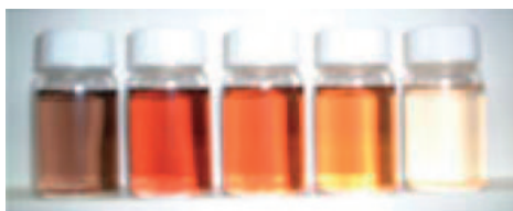
Figure 22. Photographs of THF solution of SA-stabilized Fe/Cr-CN-Co MCNPs. The ratio among the transition metals in synthetic solution was set as Fe:Cr:Co = 1:0:1, 3:1:4, 1:1:2, 1:3:4, and 0:1:1 from left to right in the figure (Ref. 57).
